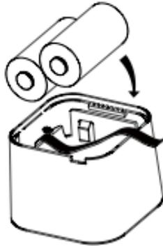
**Note:** MultiSensor 6 can be powered by a single CR123A, though batteries will require changing more frequently. If powering your MultiSensor 6 with a sole battery, insert it into the battery holder marked 1.
