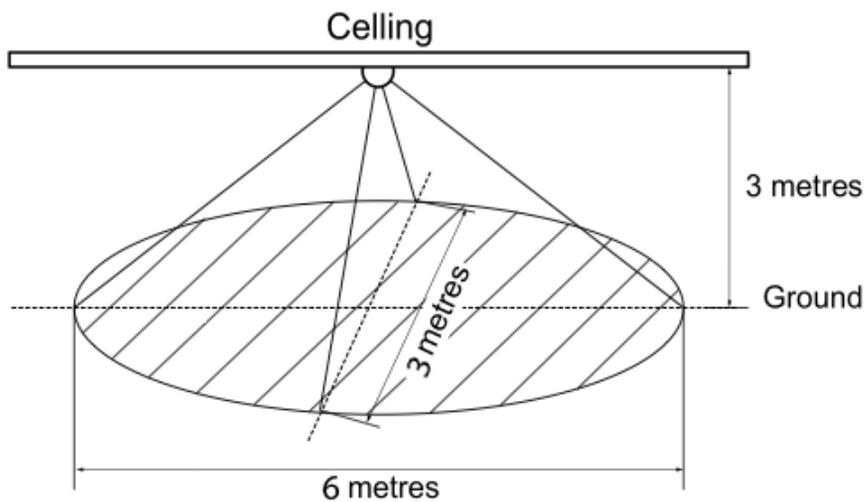
If installing MultiSensor 6 in a corner where the wall meets the ceiling it can take measurements within a 2.5 x 3.5 x 5 metres / 8 x 11 x 15 feet range:
